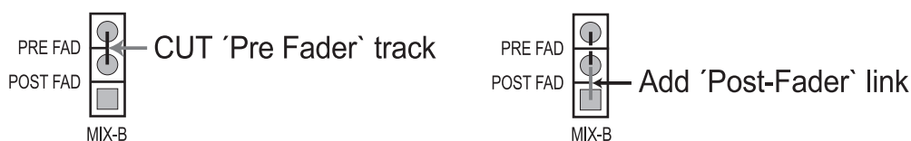
Fig. 24.2: Modifications MIX-B source > post fader
